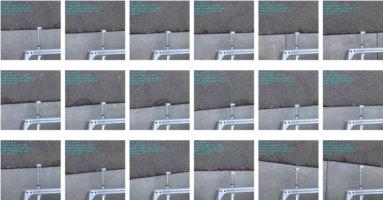
Figure 3-27 Test field at UC Davis. First row is the low amplitude maneuvering, second row is an example of medium amplitude maneuvering, and last row is the example of high amplitude maneuvering
