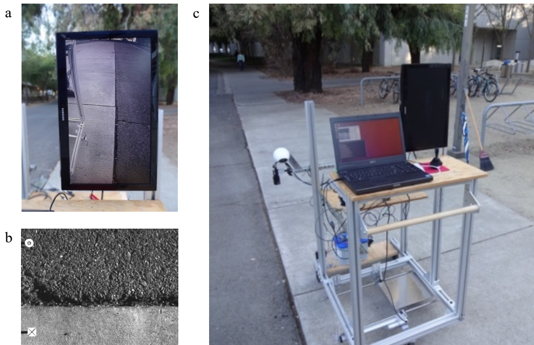
Figure 3-17 Second round of laboratory data collection setup at UC Davis: a) Leading-view camera, b) Sample of collected image of longitudinal crack with guidance labels, and c) Testbed view during image collection
