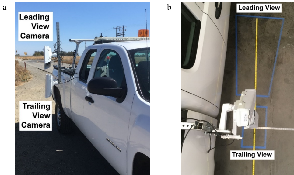
Figure 3-3 Installed positions of Leading and Trailing View cameras, a) Front-right perspective, and b) Top perspective
