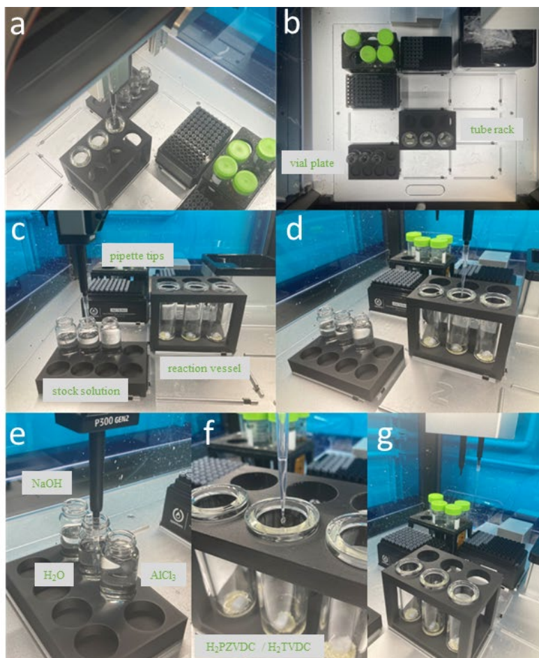
Figure 6.7 The execution of a task involving the preparation of a solvent mixture. This task, thoughtfully designed by Deng, utilizes the code illustrated in Figure 6.6 with no further modification from human user.
