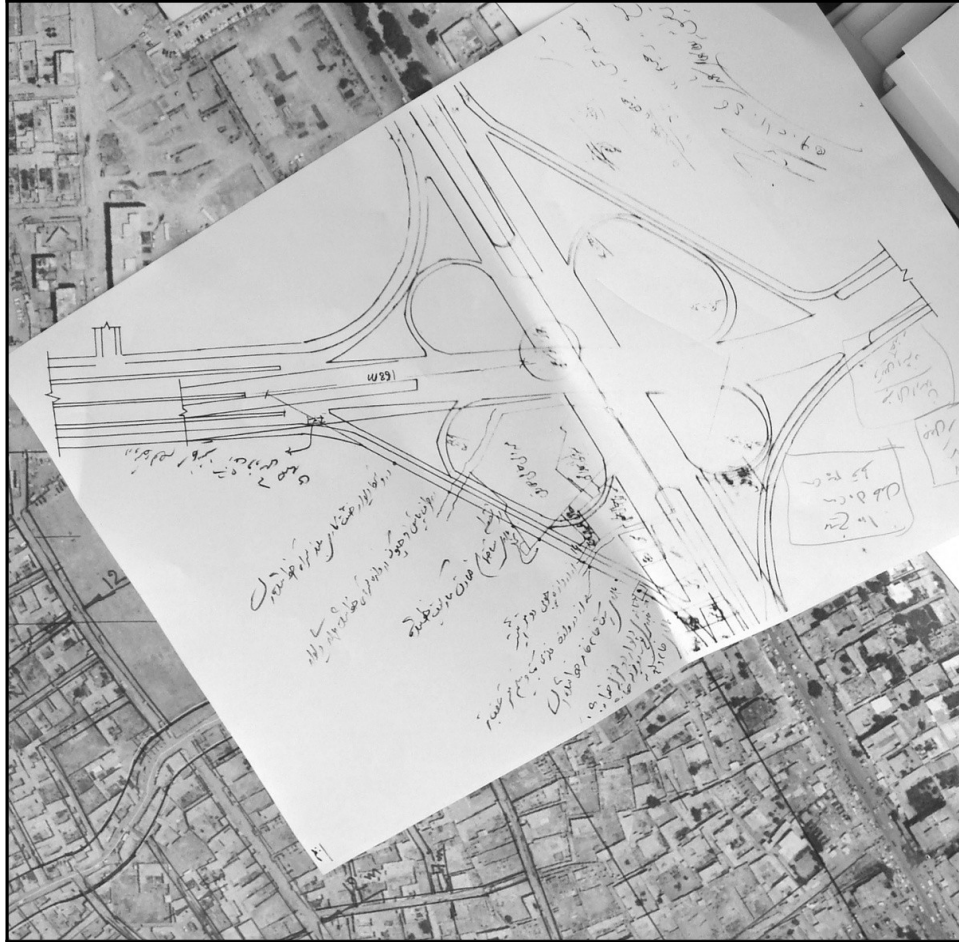
Figure 4.28. Cloverleaf overpass design overlaid on satphoto of Kota-e Sangi intersection, western Kabul (author, 2007). Road-widening and demolition work for this urban freeway interchange was already being implemented by the Municipality in 2007.
