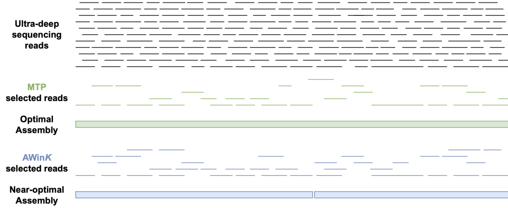
Figure 4.3: Problem formulation. Given a dataset of ultra-deep sequencing reads (top), AWinK selects a subset of reads that when given to hifiasm, it will produce a contiguous and complete de novo assembly (bottom); if the positions of the reads were known, the minimum tiling path (MTP) is the smallest subset of the reads that can be assembled to a complete genome (middle)
