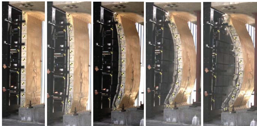
Figure 2.23: Response of CMU wall retrofitted with polyurea catcher system [27].
