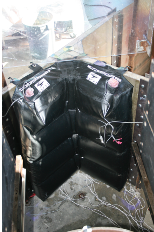
Figure 3.91: Water bladder with rotated baffles used for Composite Joint Test 4.
