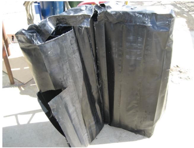
Figure 3.47: Post test photo of bladder from Surrogate Joint Test 2.
