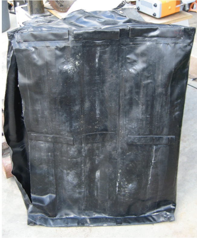
Figure 3.39: Post test photo of bladder from Surrogate Joint Test 1.
