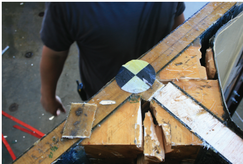
Figure 3.88: Photo of post test damage in Composite Joint Test 3.
