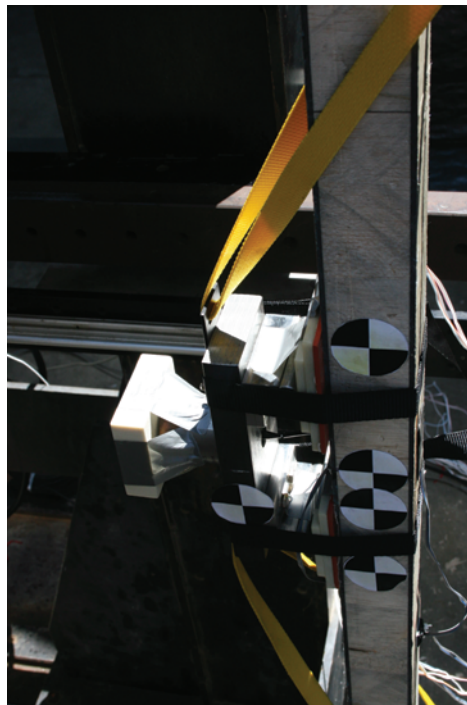
Figure 4.11: Impact plate assembly for Dynamic Bend Tests.
