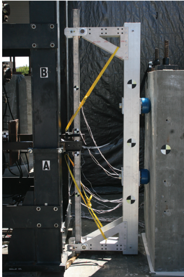
Figure 4.9: Blast Simulator configuration for Dynamic Bend Tests.
