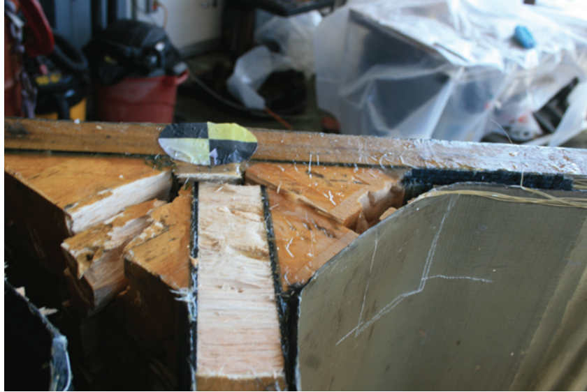
Figure 3.89: Photo of post test damage in Composite Joint Test 3.
