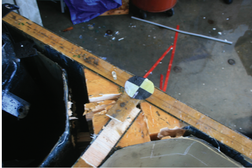
Figure 3.87: Photo of post test damage in Composite Joint Test 3.
