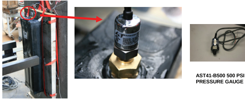
Figure 3.27: Bladder mounted pressure gauge.
