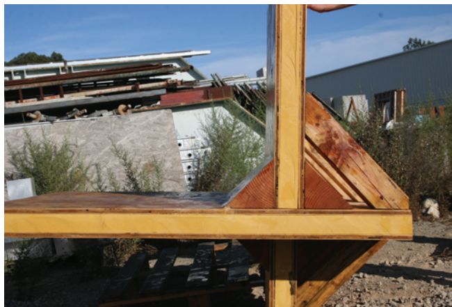
Figure 3.28: Plywood and structural foam surrogate sandwich specimen.
