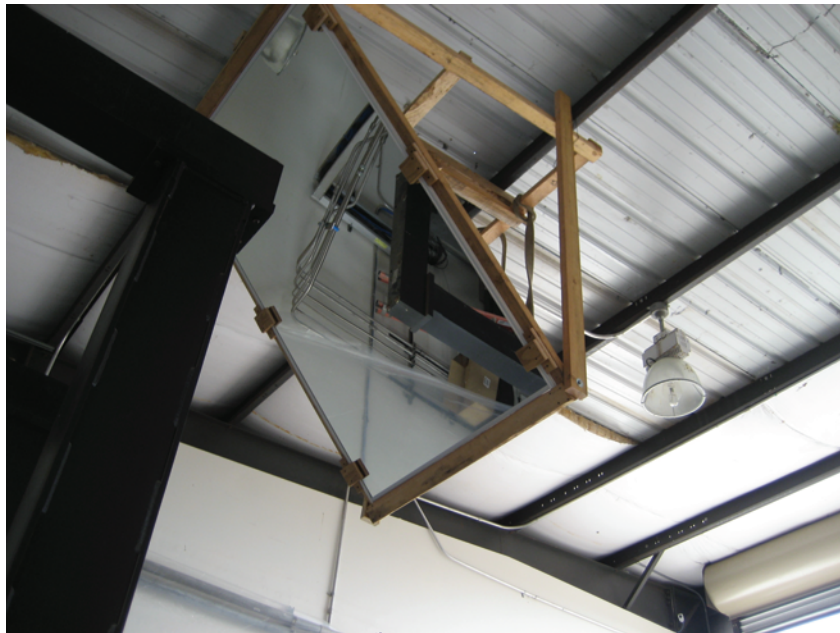
Figure 3.34: Photo of overhead mirror used for live video.
