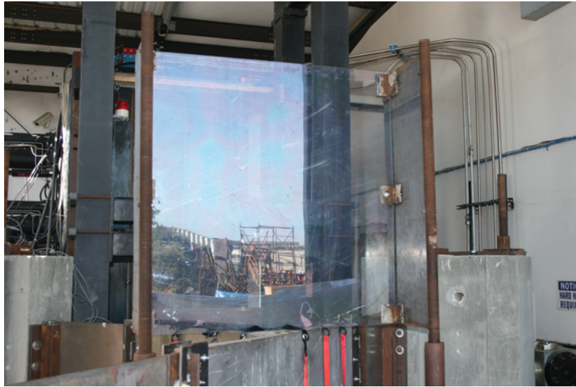
Figure 3.90: Water shield used for Composite Joint Test 4 and 5.
