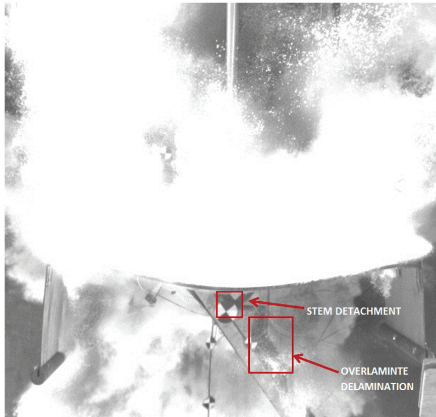
Figure 3.103: Damage progression in Composite Joint Test 5 @ t = 114.5 ms.
