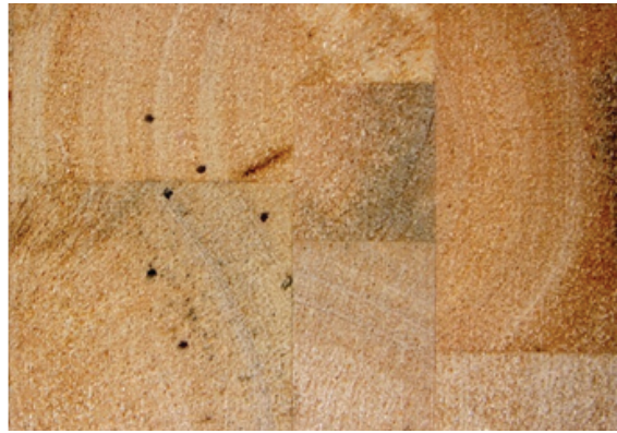
Figure 2.27: Typical balsa panel construction.
