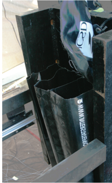
Figure 3.7: Photo of typical vertical internal baffles used to control water flow within the bladders and provide additional structural reinforcement.
