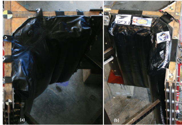
Figure 3.80: Comparison of bladders for Composite Joint Test (a) 3 and (b) 2 .
