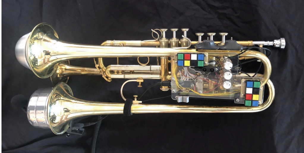
Image 1.5: Ben Neil's Mutant Trumpet 4. "Version 4 includes 16 switches, 2 X/Y joysticks, 5 potentiometers and 2 Infrared motion sensors for a total of 28 onboard controllers. The new instrument utilizes the STEIM RoSa software with a Max control interface along with Ableton Live. Version 4 made its debut in the premiere performance of Fantini Futuro at Roulette in Brooklyn, NY in September 2019"
