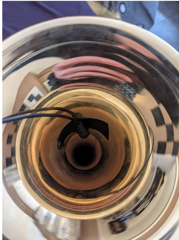
Image 3.1: Lavalier microphone placed on the inside and top of the bell for Althing I
