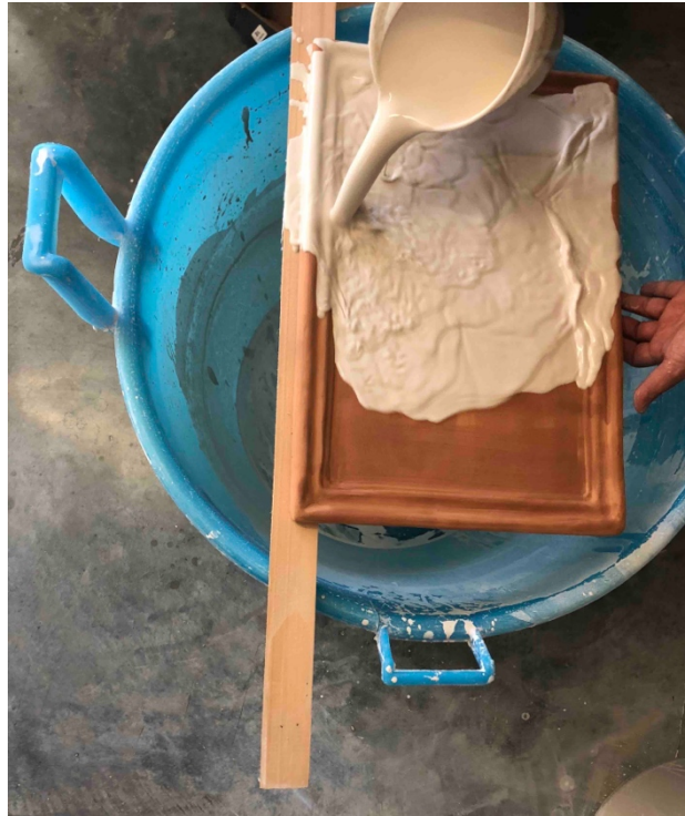
Fig. 2.5. Application of the white tin-glaze. Photo from course at Scuola d'arte Ceramica Romano Ranieri, Deruta, 2018.
