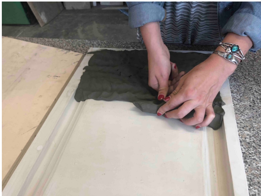
Fig. 2.3. Clay hand-pressed into plaster mold. Photo from course at Scuola d'arte Ceramica Romano Ranieri, Deruta, 2018.
