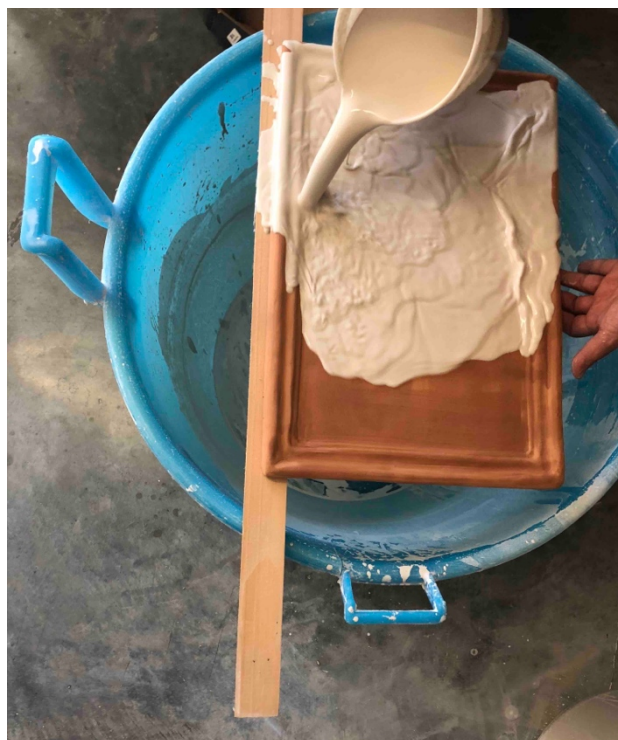
Fig. 2.5. Application of the white tin-glaze. Photo from course at Scuola d'arte Ceramica Romano Ranieri, Deruta, 2018.
