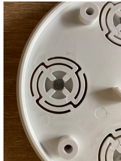
Figure 2-6. Sensor detail. Spring mechanism and metal insert on inside of bottom scale plate.
