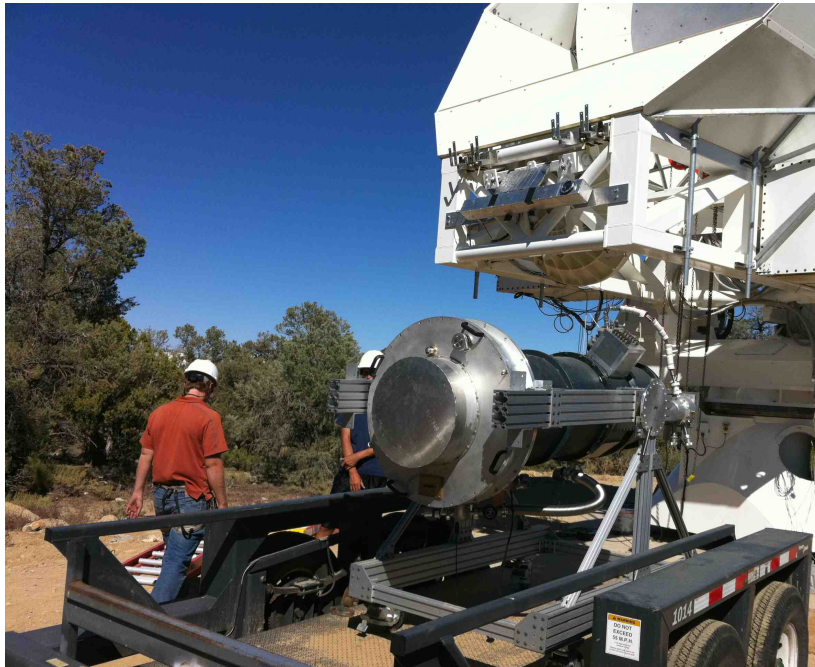
Figure 6.3: A photo taken by Prof. Brian Keating of the POLARBEAR receiver as it is being removed from the HTT at the end of the 2010 engineering run.
