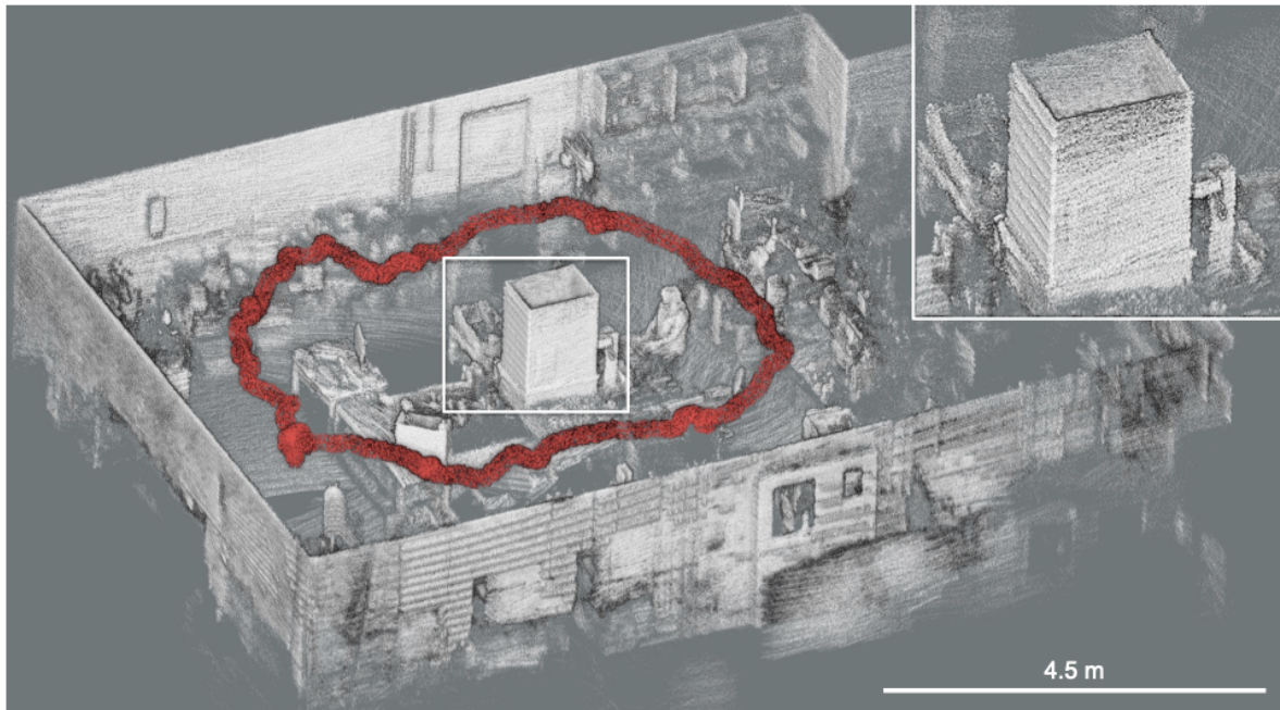
Figure 2.6: Point cloud of laboratory scene with zoomed inset showing individual point cloud points which comprise the column in the scene
