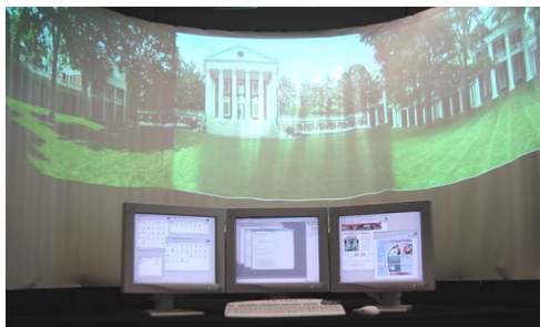
Figure 1. – The InfoCockpit uses multiple monitors to provide “location” cues and ambient visuals with three-dimensional sounds to create “place” cues.
