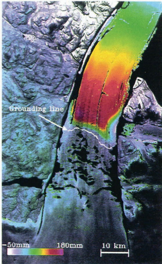
Fig. 3. Tidal displacements (color-coded between -50 and 180 \text{ mm} and modulated by the radar brightness for display purposes), and hinge line (continuous white line) of Petermann Gletscher. Dark patches indicate areas with no interferometric data.
