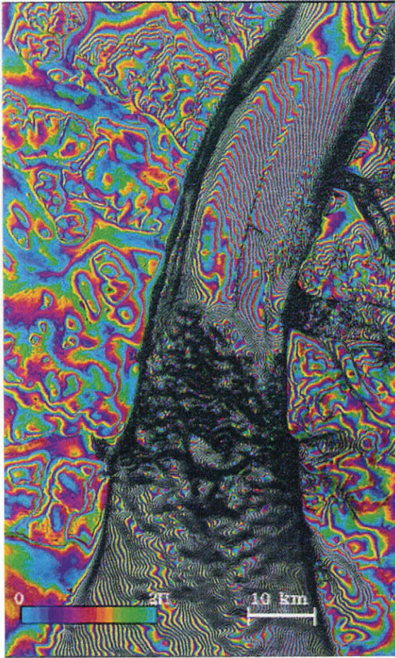
Fig. 2. Flattened interferogram combining orbits 3205 and 3248, with a color intensity modulated by phase coherence. Dark areas indicate low phase coherence.
