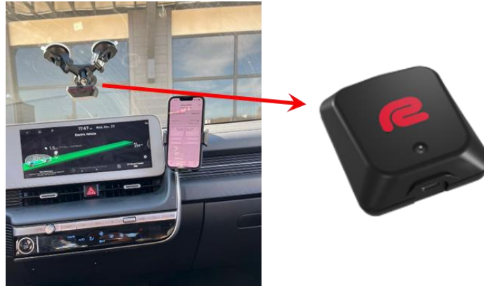
Figure 5 Racebox GPS mounted on test vehicle
