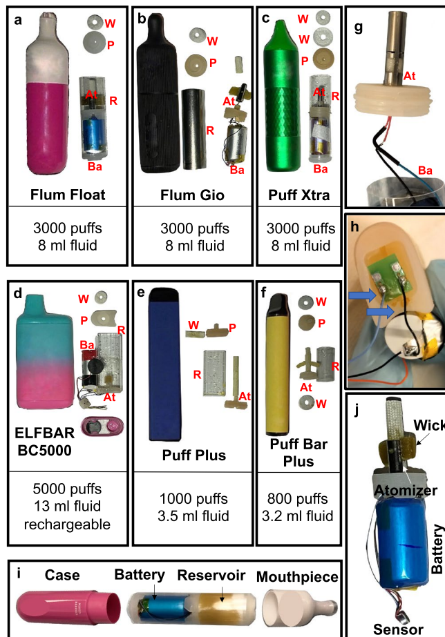
Figure 1. Dissections of six disposable ECs. (a) Flum Float, (b) Flum Gio, (c) Puff Xtra Limited, (d) ELFBAR BC5000, (e) Puff Plus, and (f) Puff Bar Plus. (a–f) show the EC before dissection and the battery and tank/atomizer after removal from the case. (g) A zoomed image of a Flum Float atomizer. (h) ELFBAR BC5000 showing signs of leakage (blue arrows) after 65 puffs. (i) Flum Float disassembled before dissection and (j) Battery and atomizer component of Flum Float after dissection. At—Atomizer, Ba—Battery, R—Reservoir, W—Washer, P—Plug.
