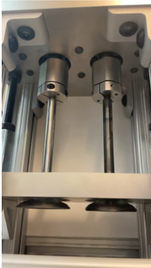
Figure F.3: Image of engine valves and adapters installed on the valvetrain test stand.
