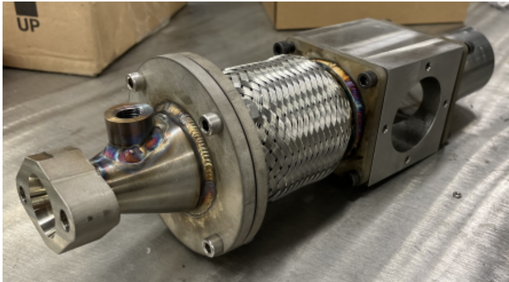
Figure C.2: Custom exhaust pipe with in-line exhaust sensor module body.
