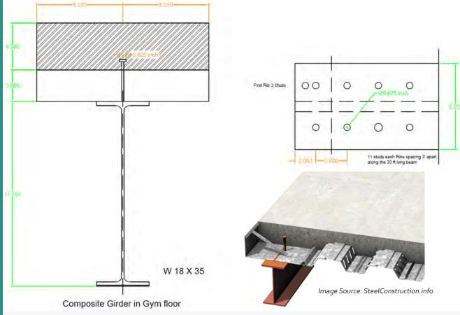
The gym floor utilizes Composite Decking, which is a popular construction technology in the industry today. Our composite beams consist of a 3.5-inch deep 4ksi normal weight concrete section and a W18 X 35 section steel with eleven 5/8 inch diameter studs along the 33 ft beam. By combining these two sections, the composite beams provide increased strength, stiffness, and load-carrying capacity compared to single material beams.
