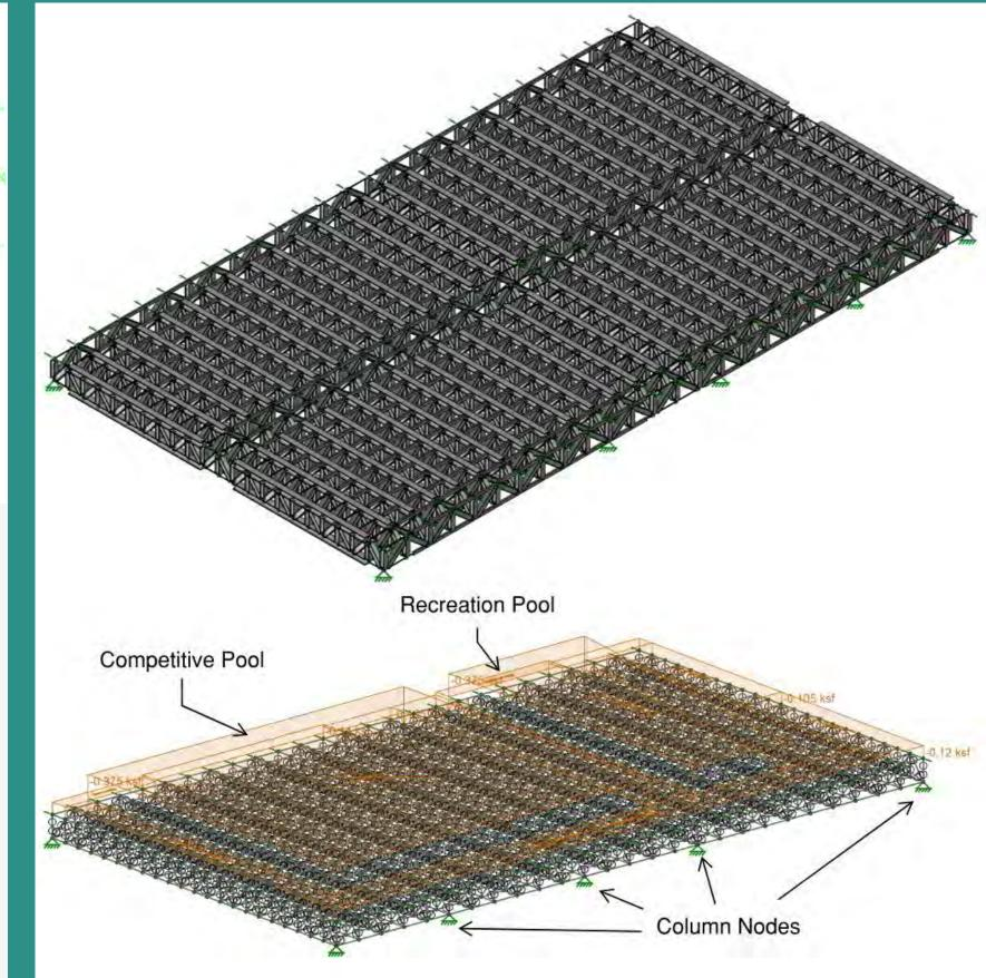
Ten columns are placed within the building to support loads sustained by the rooftop, indoor basketball gym, and parking garage. Given the construction set drawings, we arranged column locations in areas that optimized space, material costs, and aesthetic appearance. Structural elements on the roof account for load factors used to find the force transferred to the columns. Moment demand was calculated using W36x16o steel columns.
