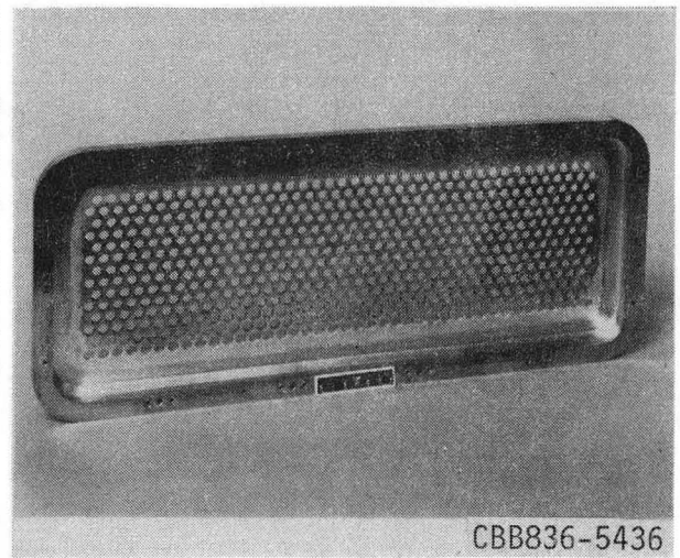
Fig. 13 Electrode of the four-electrode, 80 kV, 13 cm x 43 cm long-pulse ORNL accelerator.
