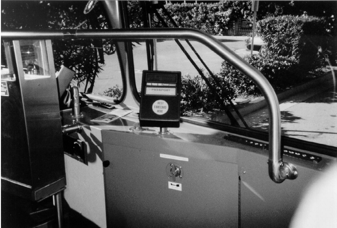
Figure 2.5a FareTrans VMS Passenger Transaction Unit Installed on a SCAT Bus
