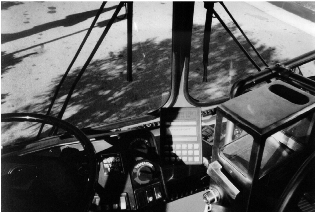
Figure 2.5b FareTrans VMS Driver Interface Unit Installed on a SCAT Bus
