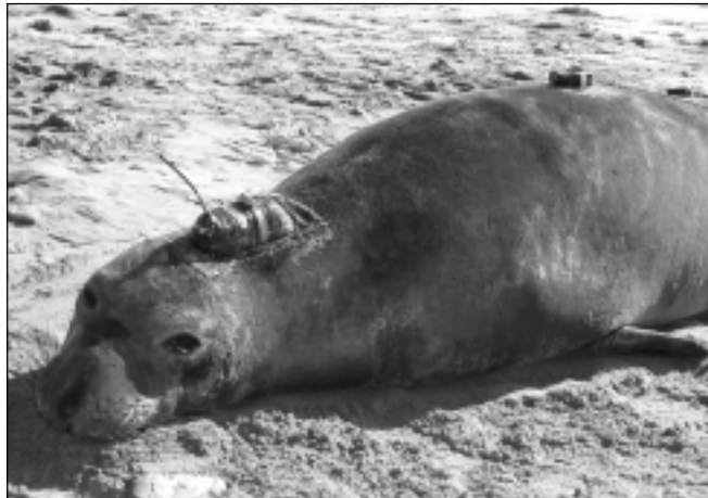
This female elephant seal, fully outfitted with a head-mounted platform transducer and time-temperature-depth recorder (TTDR) attached to her back, is a participant in studies at Año Nuevo that aim to find out where she and her friends go, how they get there, and what they do. Photo by Dan Costa
