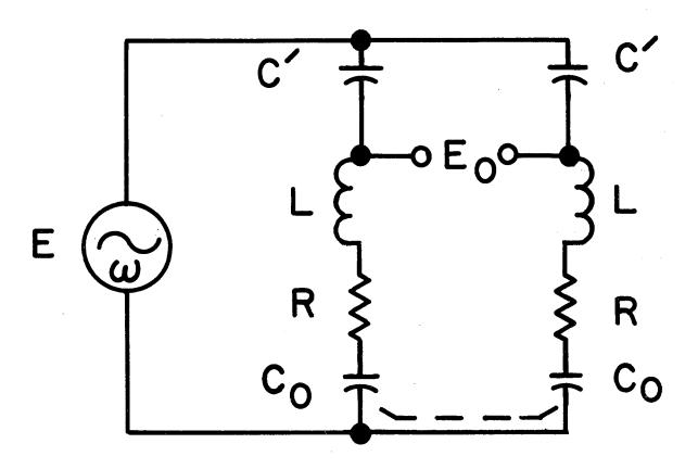
Fig. 1. Resonant-bridge network. Here E is the bridge excitation voltage, E\_0 is the bridge output voltage, C\_0 is the manometer capacitance in each leg, R is the ac resistance of L, and LC\_0 =  $1/\omega^2$ , with  $\omega = 2\pi f$  where f is the frequency.
