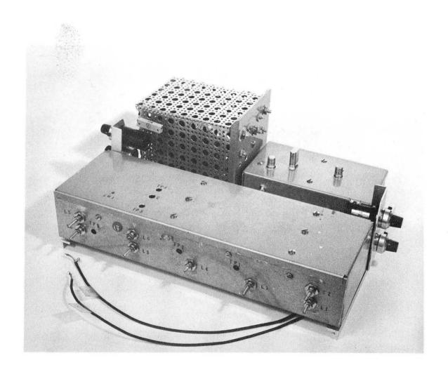
Fig. 8. Top-front view of the electronics. The remotely located pressure transducer is not shown. Construction is modular. The null detector is in the foreground. The power supply is at left rear; the generator module is to its right.
