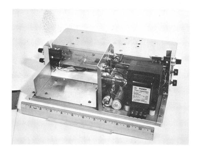
Fig. 10. Power supply, with calcaine cover removed. The generator module, normally mounted left front, has been removed to indicate the manner of mounting. Angle brackets unitizing the modules can be seen to the left and right. The power supply and generator modules are mounted on a plate formed from a cover identical to the one shown on the null detector.
