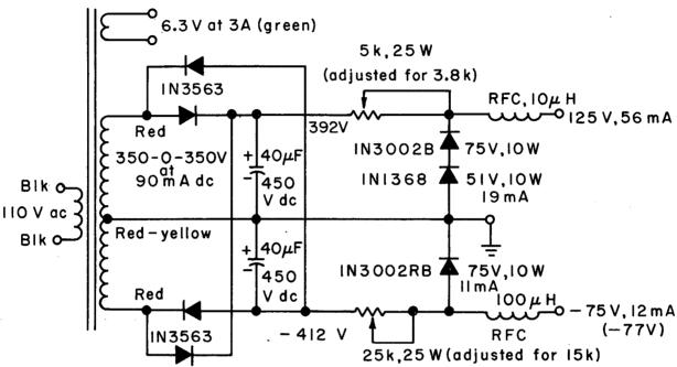
Fig. 7. The power supply. All voltages and currents were measured when operating with a Sola voltage-regulating transformer. Without this transformer, 392V becomes 453V, -412V becomes -486V, 19 mA becomes 32 mA, and 11 mA becomes 15.4 mA. The  $40\mbox{-}\mu\text{F}$  capacitors should have a 500-V working voltage if the Sola transformer is not used.
