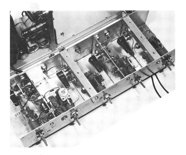
Fig. 14. Top left view of null detector, illustrating construction in detail.
