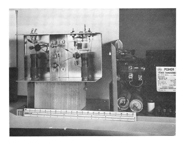
Fig. 11. Generator module tilted so that it can be viewed from underneath. The oscillator compartment is to the left, buffer at right.
