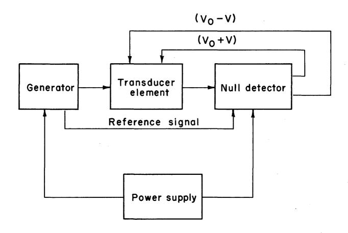
Fig. 3. Block diagram of the electrical system. Here  $V_0+v$  is the restoring voltage applied to one plate, and  $V_0-v$  is the restoring voltage applied to the other.
