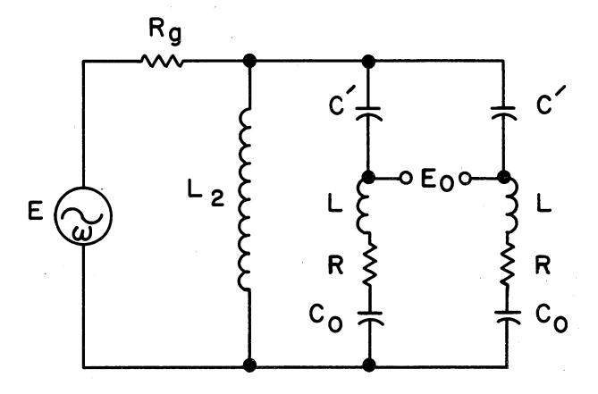
Fig. 2. Resonant bridge with matching network. Here  $R_g$  is the generator impedance and  $L_2C\,{}^\prime{=}\,1/2\omega^2$ . Other parameters are defined in the legend of Fig. 1.
