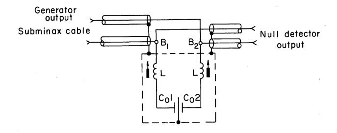
Fig. 5. Transducer element (within dashed lines). Terminals  $B_1$  and  $B_2$  connect to corresponding terminals of both the generator and the null detector. Capacitances  $C_01$  and  $C_02$  of each side of the membrane manometer are about 75 pF. Inductance L is 64 turns of No. 32 Formvar wound on National Radio Corp. form XR50.
