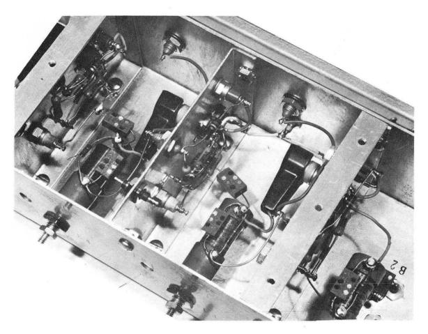
Fig. 15. Inner compartments of the null detector viewed from above and right.
