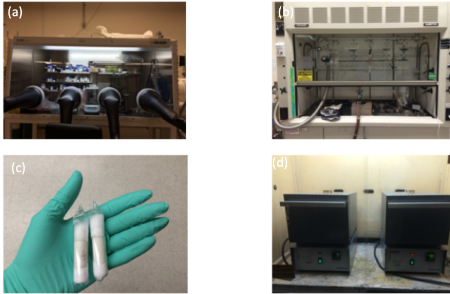
Figure 3.1: (a) A glovebox filled with Ar gas where most of the materials are kept. (b) The apparatus for evacuating and sealing quartz tubes. Tubes are connected to a pumping line, evacuated, and sealed off using a blow torch. (c) Sealed quartz tubes, with the starting materials held inside the \text{Al}_2\text{O}_3 crucibles. (d) Box furnaces that can reach 1100^\circ\text{C} .
