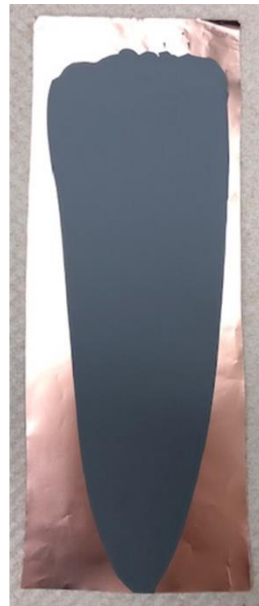
Figure 2. 1 Electrode preparation for LFP casted on the Al foil (left) and LTO casted on the Cu foil (right)
