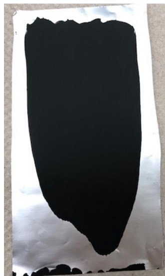
Figure 2. 1 Electrode preparation for LFP casted on the Al foil (left) and LTO casted on the Cu foil (right)
