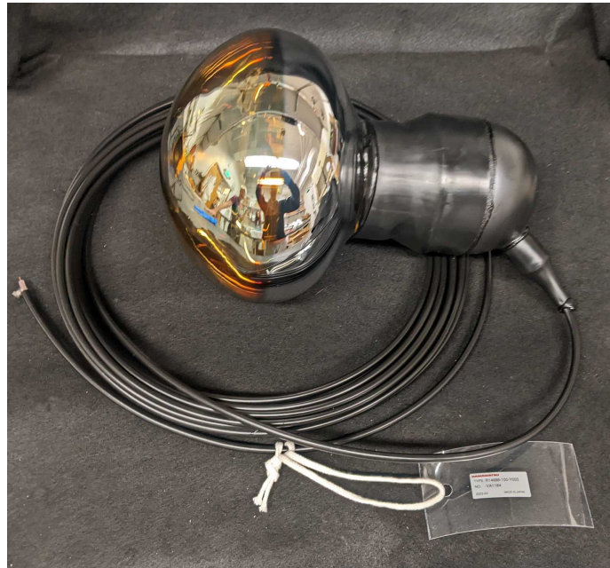
Figure 1. The R14688-100 PMT with the black water-proof potting and the 20 meter SHV cable.
