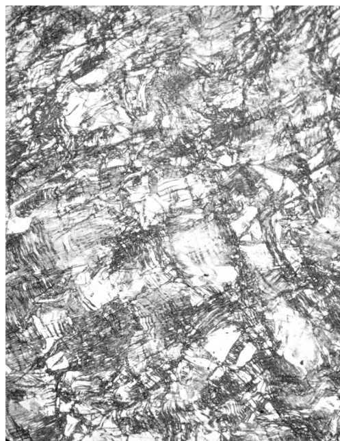
FIGURE 8.29. Microstructure M21, etched with K_2Cr_2O_7 + EthFeCl_3 ; magnification 400X. Photograph by Samuel Nash.
