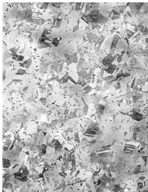
FIGURE 8.23. Microstructure M16, etched with K_2Cr_2O_7 + EthFeCl_3 ; magnification 200X. Photograph by Samuel Nash.
