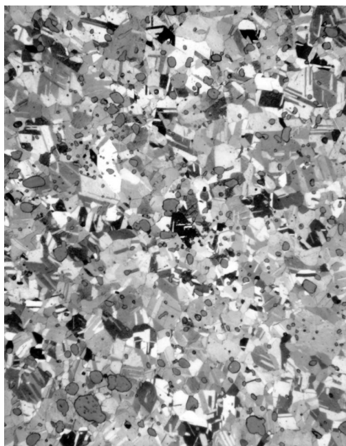
FIGURE 8.27. Microstructure M18, etched with K_2Cr_2O_7 + EthFeCl_3 ; magnification 400X. Photograph by Samuel Nash.
