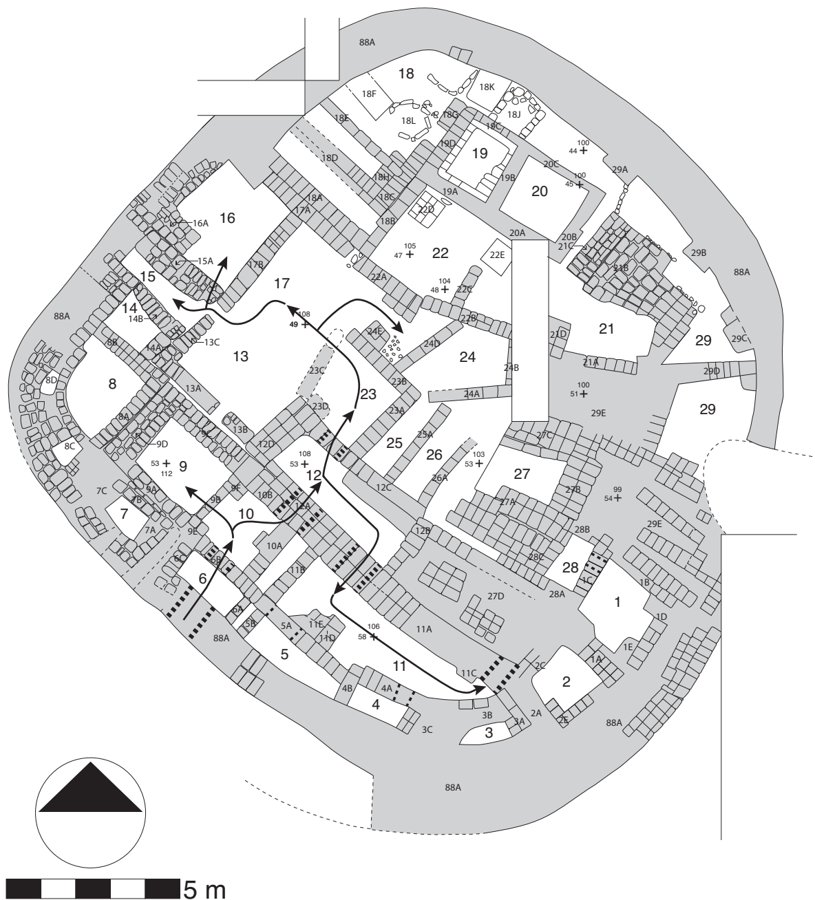
FIGURE 2.17. Level 4 Round Building, with routes of access in south and west. Corbel arched doorways indicated by thick dashed lines; windows indicated by thin dashed lines. Illustration prepared by Harley King.
