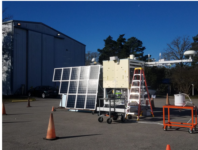
Figure 3.10: The integrated COSI detector, telemetry, and power system in the 2020 Balloon Campaign.
