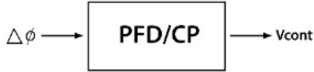
Figure 12: Input and output of Phase Frequency Detector and Charge Pump
