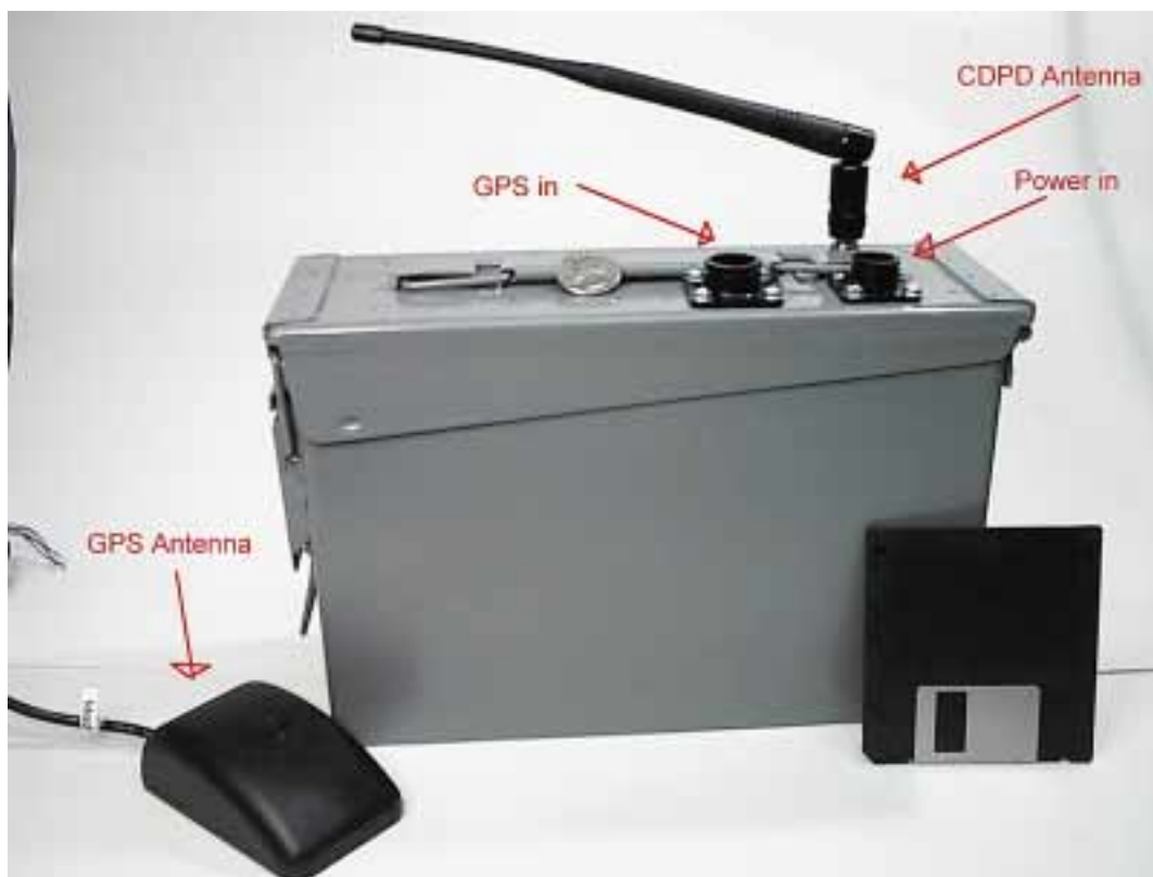
Figure 1: Extensible data collection unit, complete with GPS antenna and cellular data modem antenna.
