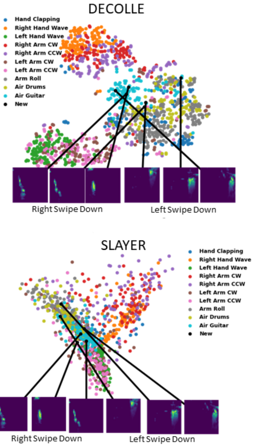
Figure 5.6: A T-SNE plot DVSGesture dataset and real-world gestures using the convolution layer output of SLAYER and DECOLLE models.
