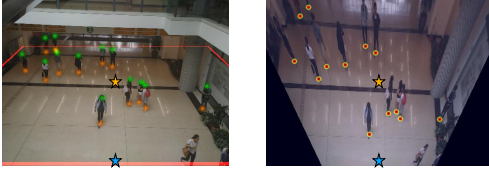
Figure 3: Example ground-truth heatmaps overlaid on the input image. Left: IV maps, with heads in green and feet in red. Region of interest is bounded by a red perspective box. Right: BEV location map. Centers and bottom centers of heatmaps are aligned.
