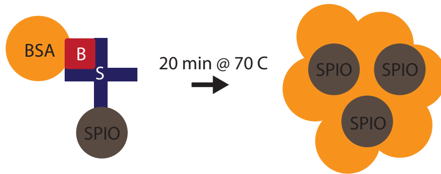
Figure 2.1: Preparation of MAA-SPIOs. Biotinylated albumin is conjugated to streptavidin-functionalized SPIOs, then heated with stirring to form macroaggregates. B = biotin, S = streptavidin, BSA = bovine serum albumin, SPIO = superparamagnetic iron oxide nanoparticle.
