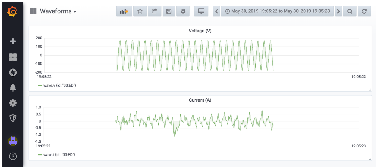
Figure 3.6: Voltage and current waveforms at Influx, viewed on Grafana. The ESP32 can connect to a PowerBlade, retrieve calibration values, and read 1260 values of voltage and change of current—representing 0.5s of data—from the raw sample service. The gateway then adjusts the data using the calibration figures, calculates the real-time current values, timestamps every point, and sends the final voltage and current waveform data to an Influx database via HTTP POST. The entire process takes around 82s.
