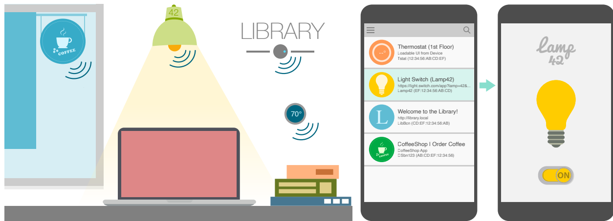
Figure 2.2: Browsing model for device interaction. Smart devices (light bulb, thermostat) and beacons make their presence known by broadcasting information about themselves. The browser, which can run on a smartphone, scans the local vicinity and displays to the user a selection of available user interfaces for nearby devices. When the user makes a selection, the interface for the chosen device is opened from a specified location hosted locally or online, presenting a user interface that can facilitate direct interaction with the device using browser-extended APIs for local network communication protocols.
