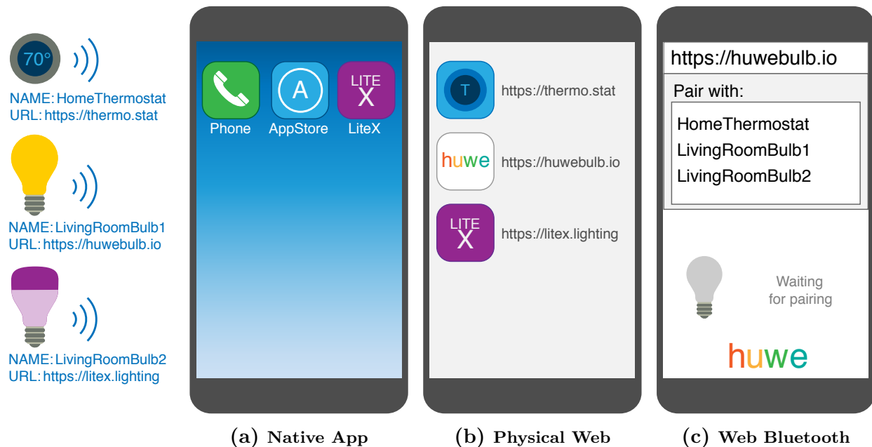
Figure 5.1: Native App, Physical Web, and Web Bluetooth. The native app model (a) requires that a user have prior knowledge of a device and install an app to interact with it. The Physical Web model (b) allows discovery of URLs broadcast by nearby devices, but does not provide device details to the user. The Web Bluetooth model (c) requires that, once a user manually navigates to a website, the user select the device to pair with the website. Even if, perhaps, (b) and (c) are used together, the user would still need to identify the correct device without information on which device pointed to the site.
