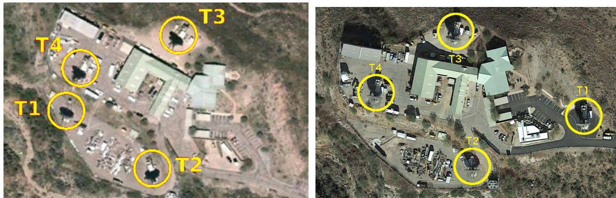
(a) Original arrangement of telescopes in the V4 epoch. (b) Satellite image of telescopes after T1 was moved to a more symmetric position.
