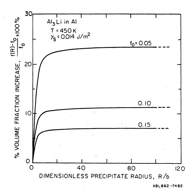
Figure 6 Cumulative change in precipitate volume fraction during coarsening for Al<sub>3</sub>Li precipitates in Al
