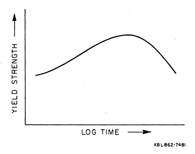
Figure 1 Schematic aging curve
