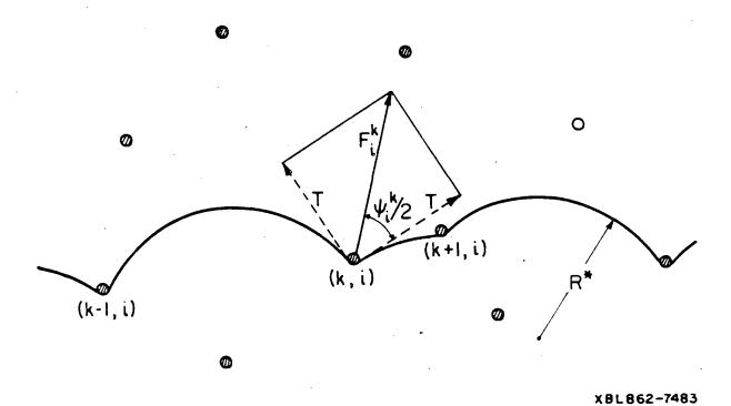
Figure 2 Dislocation bow-out under stress between point obstacles
