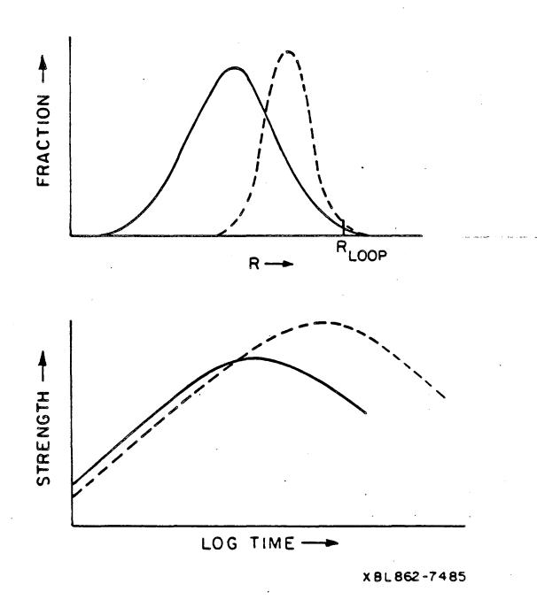
Figure 5 Advantage of a narrow precipitate size distribution
