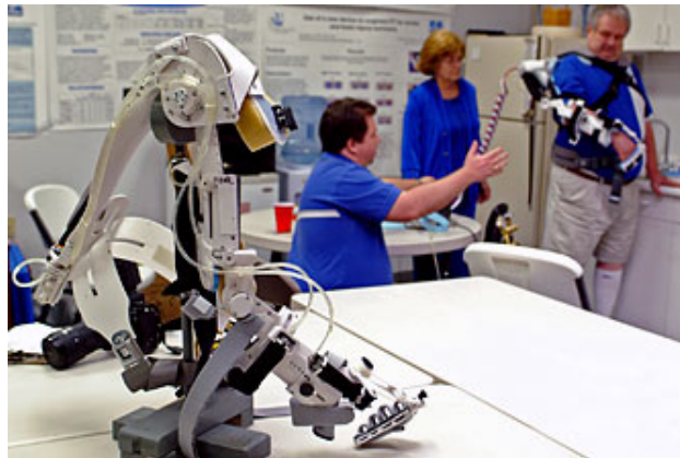
Figure 2.2: Wearable RUPERT exoskeleton for arm with hemiparesis.
