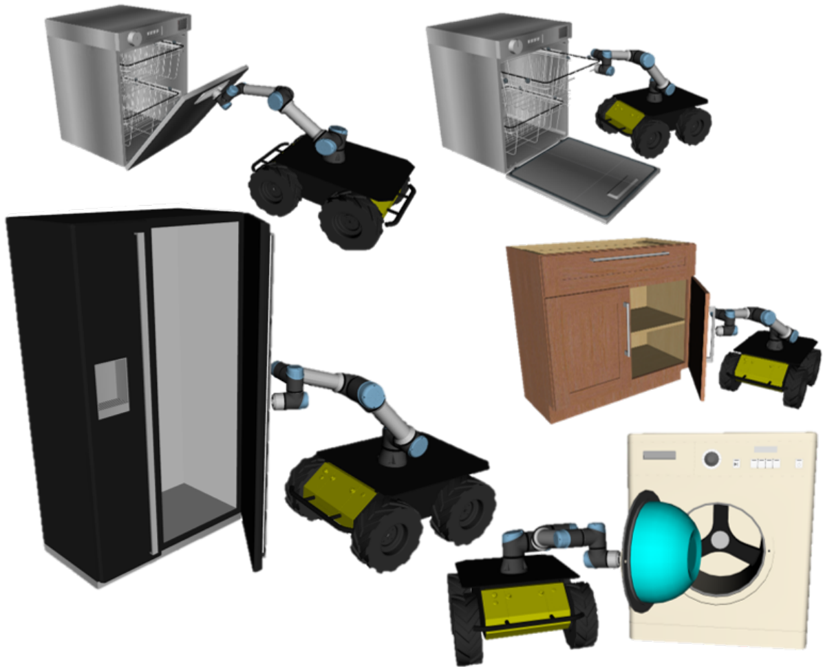
Figure 3.2: Diverse interactions a service robot needs to perform in a household environment. By abstracting the objects’ kinematic structures and forming a VKC, a service robot can plan and act more efficiently with improved foot-arm coordination.
