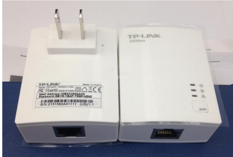
Figure 40. PLC adapter pair for PLC communication design
