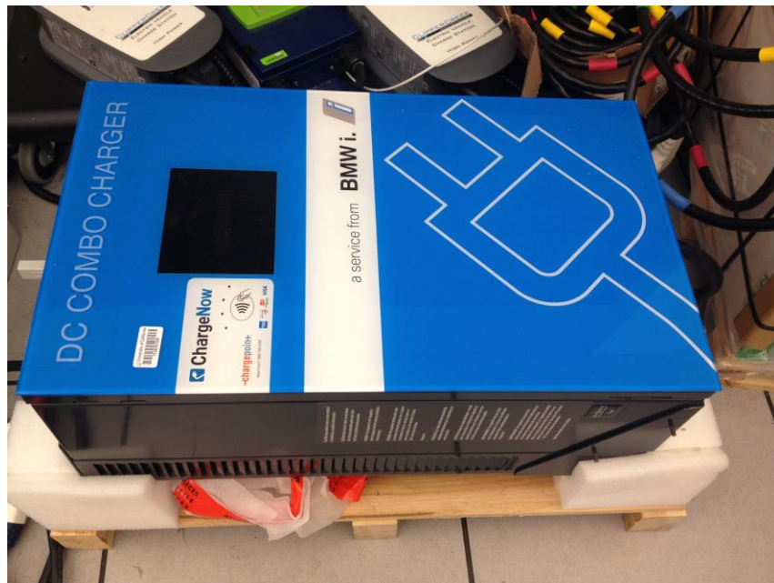
Figure 39. DC combo charger for level 3 fast DC charging
