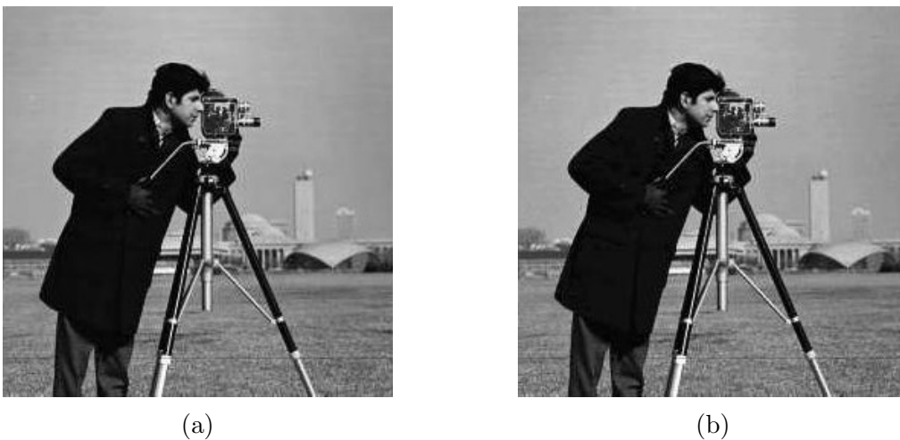
Figure 4.1: Full (a) and approximate (b) compressed images where PSNRs are 31.74 and 31.52 respectively
