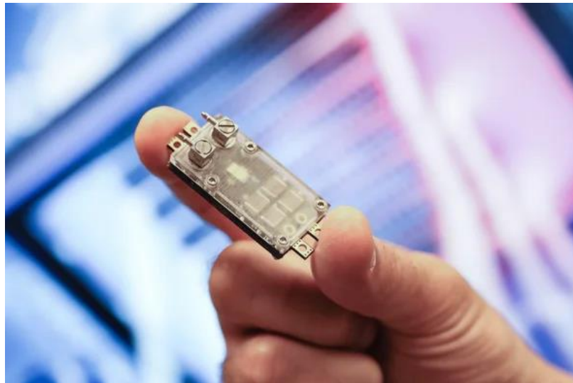
Figure 1-3 Image of a chip with an integrated microchannel cooling system developed by Swiss Federal Institute of Technology in Lausanne (This image is available in the public domain, Credit: Copyright © Alain Herzog EPFL).
