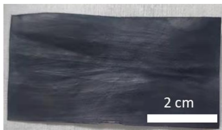
Figure 2.9. Photograph of a QxTh:rGO 1:5 film prepared on a graphite foil.
