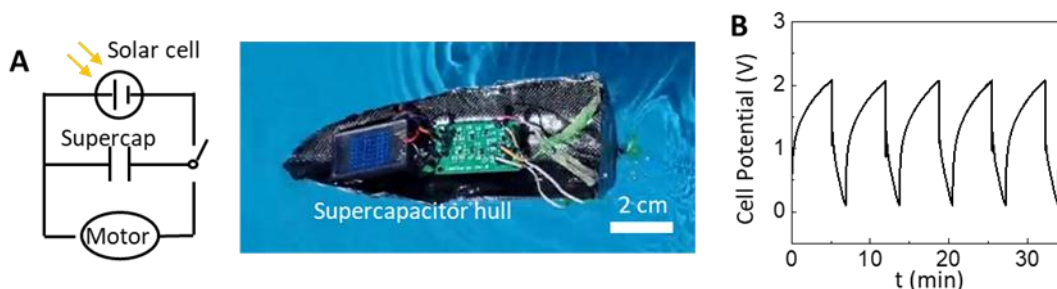
Figure 3.24. (a) A schematic and photograph of a boat model, in which the entire boat hull is a structural supercapacitor. The structural supercapacitor was charged by solar cells to power the boat motor. (b) Charging/discharging voltage at the supercapacitor terminals versus time when operating within the energy harvesting system to drive the boat motor.
