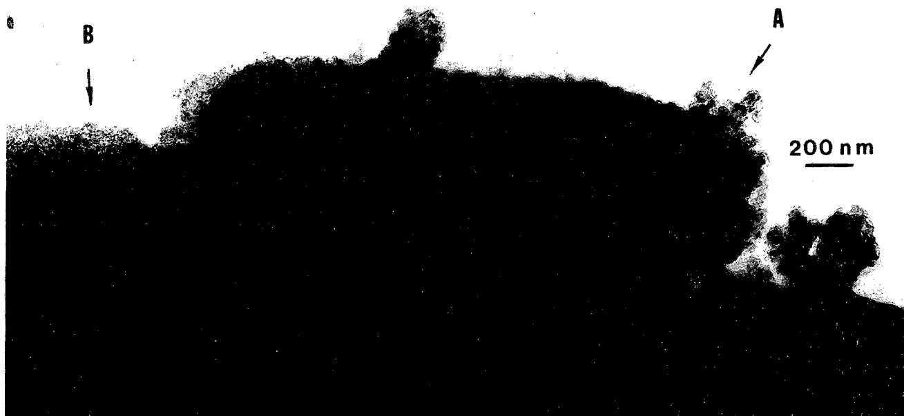
Figure 8. Low magnification image of the specimen after exposure to an intense electron beam during high resolution imaging (area A). Notice the difference between areas A and B. (XBB 847-5468a)
