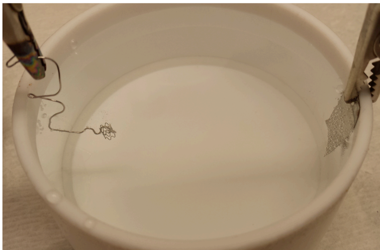
Figure 18. Anodization setup for the synthesis of the nanowell coating on Nitinol stents.
