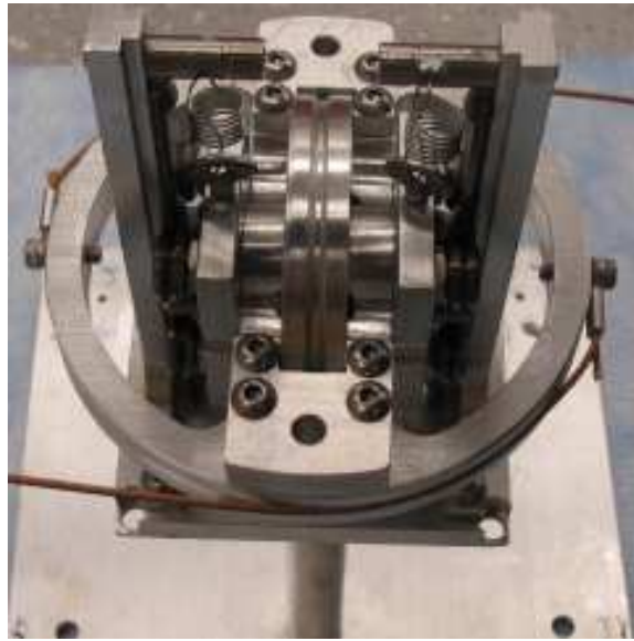
Fig. 3.3 Isometric view of a sliding ring cable driven mechanism used for pure moment testing in axial rotation (with current setup is simulating right axial rotation).
