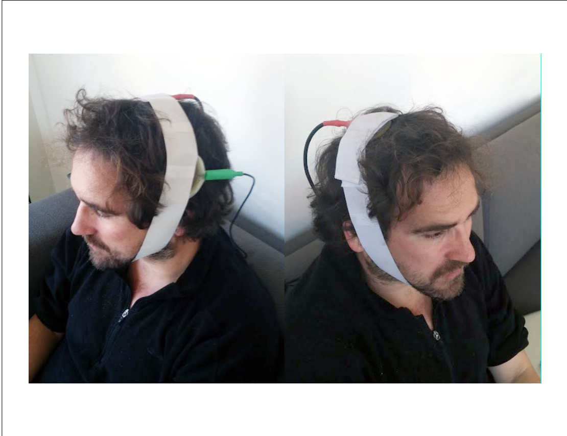
Figure 5.3. TEFS prototype plate(s) placement. The right side shows the device typical use when one plate (high voltage plate) is placed over the the user's head. The left picture shows a typical use when two plates (high voltage plate and ground plate) are placed over the user's head. In these pictures no particular parts of the user's brain has been targeted and the pictures are taken solely for the demonstration purpose while the TEFS device is not turned on.
