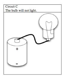
Figure 3.2. Diagram of an incomplete circuit.
