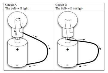
*Figure 3.1.* Diagrams of two complete circuits. Circuit A will light the bulb while Circuit B does not.
