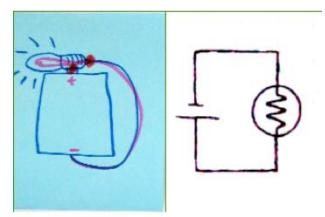
*Figure 5.6.* Iconic (left) and schematic (right) drawings of complete circuits with lit bulbs.
