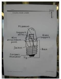
Figure 5.4. Close-up image of the "architecture of the light bulb" wall chart.
