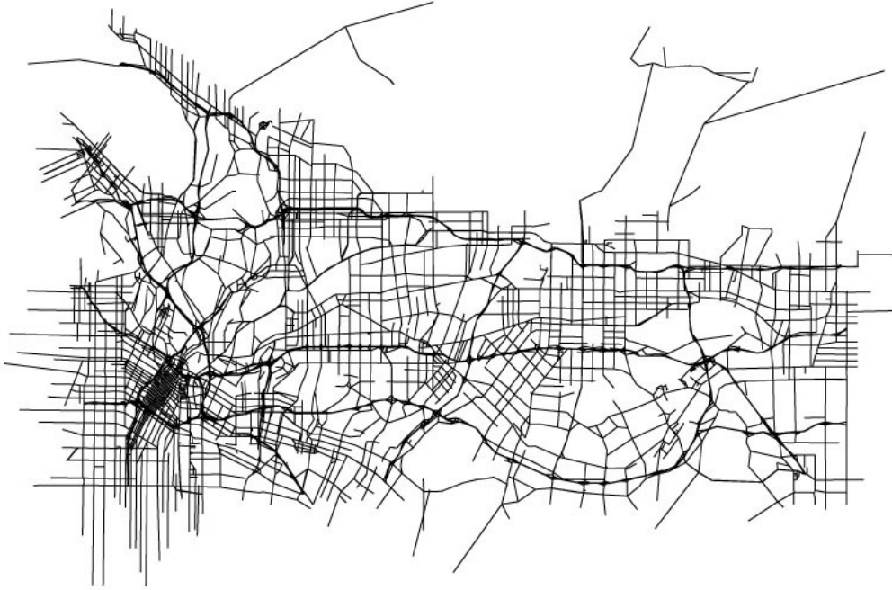
Figure 10.6: Full-scale network including highway and arterial networks of the I-210 corridor used for MATSim data generation, and for the estimation problem. See Figure 10.2 for the Voronoi tessellation model of the cellular network and the 700 origins given by the TAZ.
