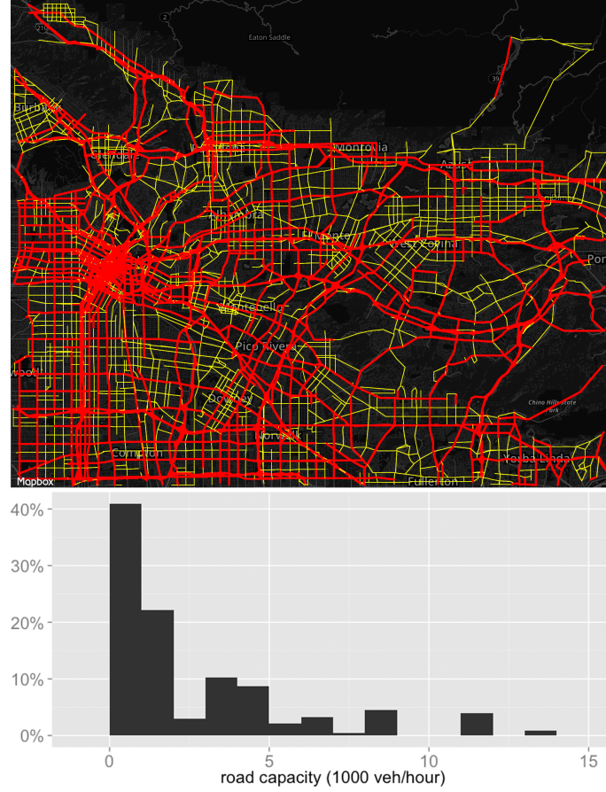
Figure 4.1: The map of Los Angeles, CA used for the present study composed of 28,376 arcs and 14,617 nodes extracted from OpenStreetMap. Information for each edge includes the free-flow travel time, length, capacity, and speed limit. Links with capacity less than 1000 vehicles per hour are considered low-capacity (in yellow) while links with 1000 vehicles per hour or more are considered high-capacity (red). The histogram of the different road capacities are shown in the bottom figure, with more than 40% of low-capacity links.
