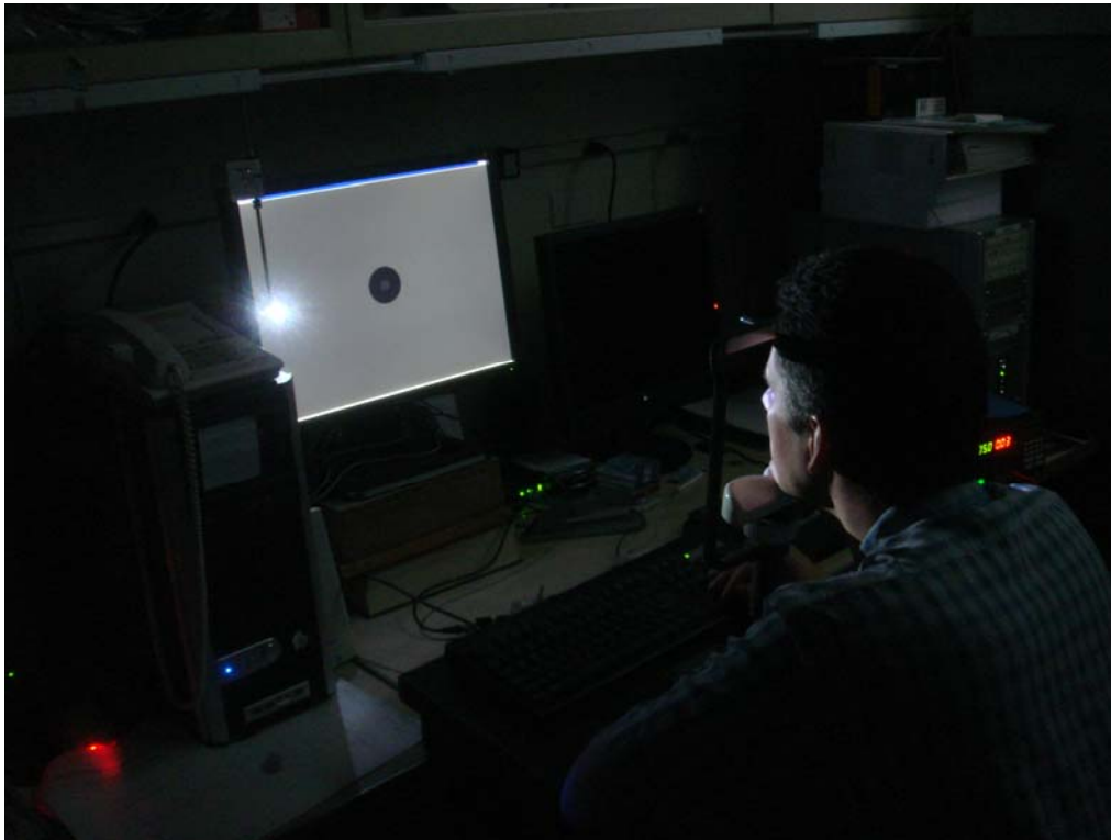
Figure 1. Photograph of the disability glare experiment task, showing the computer monitor with glare source illuminated. The observer adjusted the intensity of the disc within the annulus to threshold.
