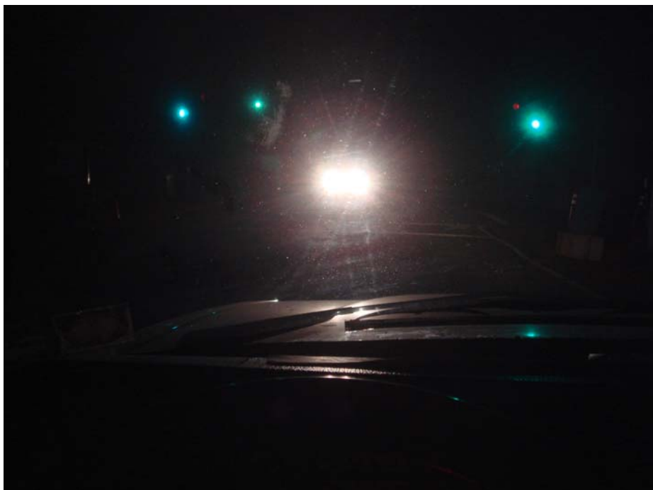
Figure 1e. Glare from headlights of opposing vehicle as seen through windshield of primary vehicle.
