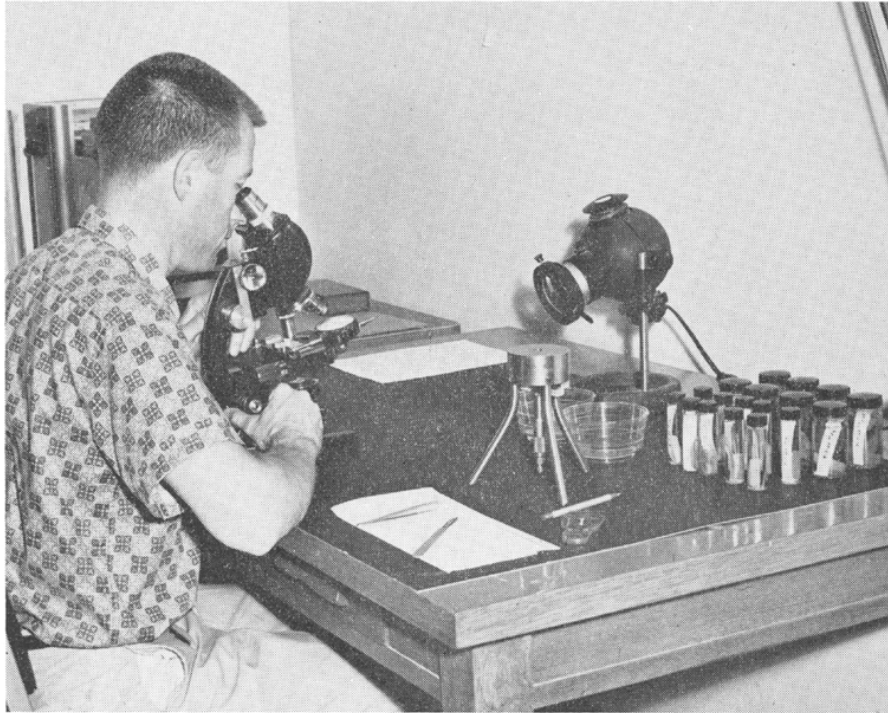
FIGURE 43. Robert A. Iselin, at the California State Fisheries Laboratory, Terminal Island, measuring albacore eggs as part of a maturity study. Note dial indicator attached to microscope, for measuring egg diameters. Photograph by Robert R. Bell.
