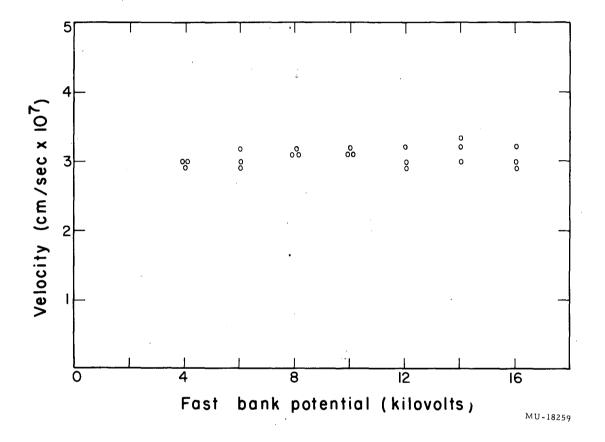
Fig. 26. Measured wave velocity vs fast-bank potential.
