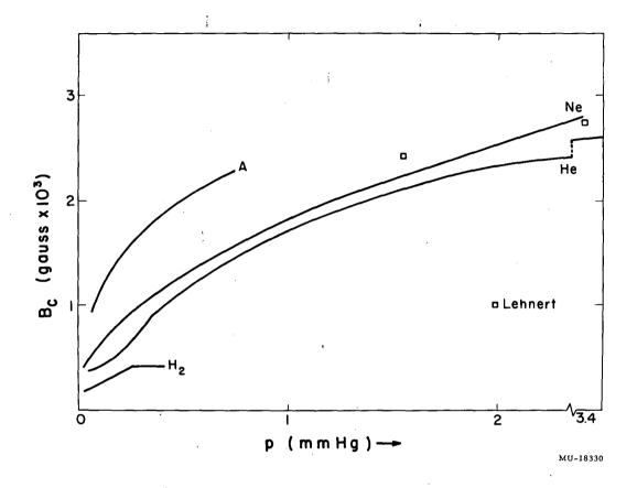
Fig. 19.  $B_c$  of electric field vs pressure, for various gases.
