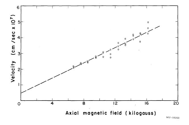
Fig. 27. Measured wave velocity vs axial magnetic field. Dashed line indicates linear dependence predicted by theory.
