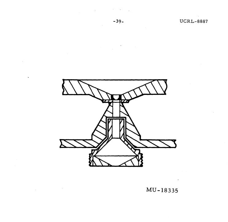
Fig. 12. Modified arc geometry, Source I, Series C.
