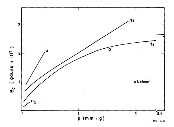
Fig. 20.  $B_c$  of 125-kc noise vs pressure, for various gases.
