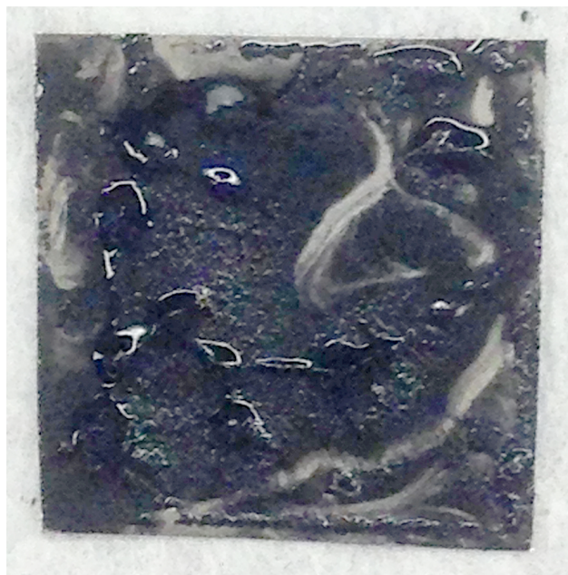
Figure 5.10: Photograph of MnO 2 electrode from cell with [1:15]1:1:5 + 0.5% water GPE after cycling.
